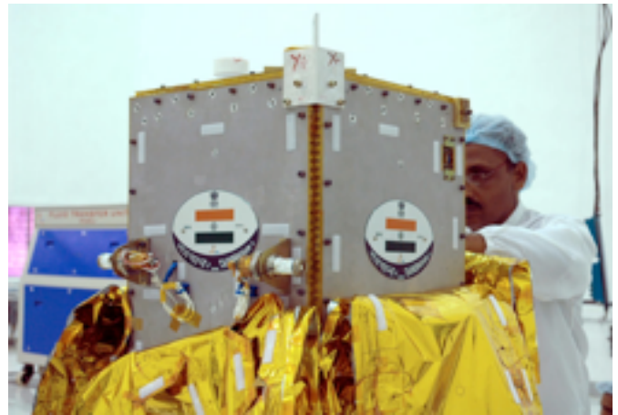
Moon Impact Probe to be released early in the mission in an attempt to splash out water vapor from a S. Pole crash site.
