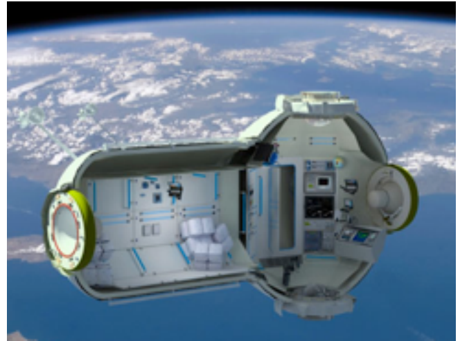
Cut-away illustration of an EA space station in orbit 11 meters long by 4 meters wide (36 x 13 ft)
