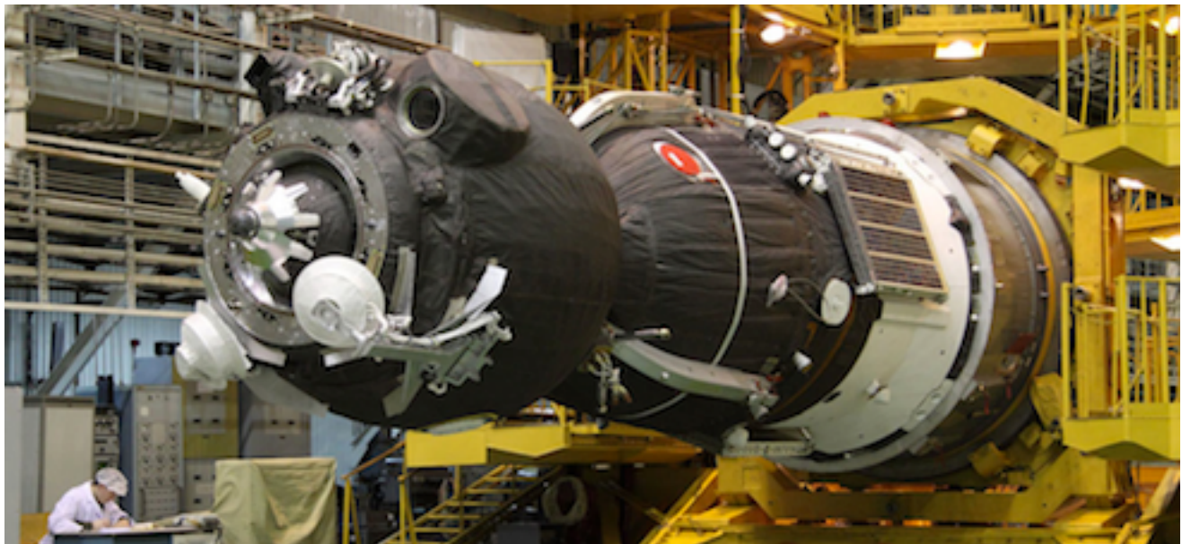
Above: a Soyuz Capsule prior to being placed in its faring on a launch rocket. See worker at lower left for an idea of scale.
