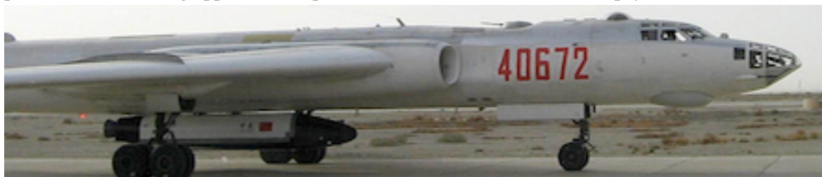
Photo of Shenlong slung below launching plane between wheels
