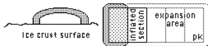
Ice-shielded surface base hanger: elevation (L), plan (R).
